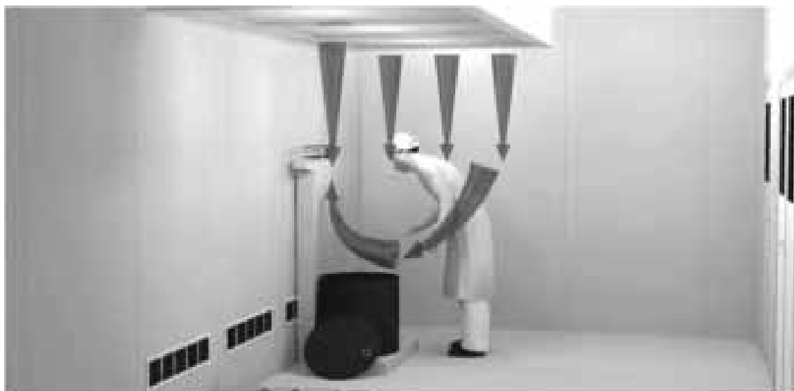
Operator subject to powder contamination due to airflow reversal in bin
