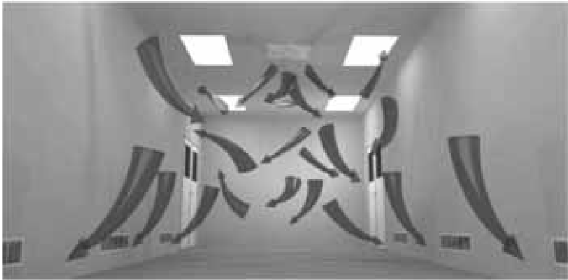
Figure 6 Turbulent dilution of dirty air
