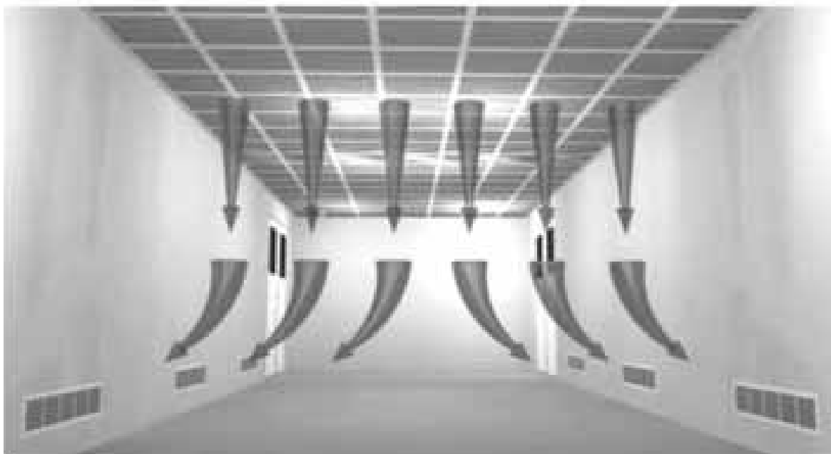
Figure 7 Unidirectional displacement of dirty air
